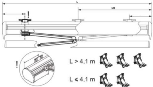
Wall brackets should be installed in spots marked by the manufacturer in the rear part of the cassette (so that they are "in the axis" of the symmetry of the arm brackets).
